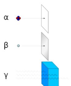
As shown in the diagram above, the different radiation materials shall be stopped by more and more dense and thick elements illustrating the penetrating power of radiation.
