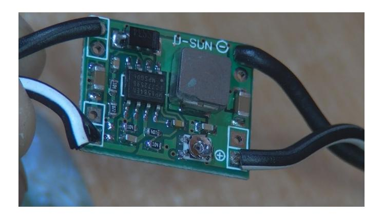
Buck 3A DC Converter Step Down Module
